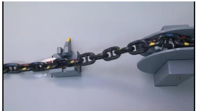
Using a crow bar, rotate the chain when loose opposite to the twist direction.
