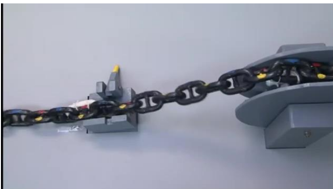
Using pads attached 1-2 meters apart depending on your ship's machinery locations, you can rotate the chain when the first pad enters the chain winch (the pad lifts the chain allowing for the rotation) and thus gradually eliminate the twist.
