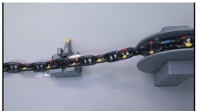
Using pads attached 1-2 meters apart depending on your ship's machinery locations, you can rotate the chain when the first pad enters the chain winch (the pad lifts the chain allowing for the rotation) and thus gradually eliminate the twist.
